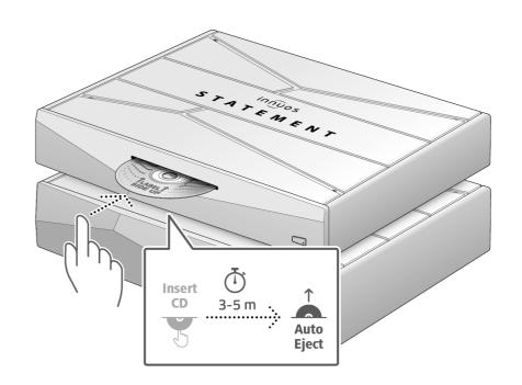
Do not push the CD while it is being drawn in as this may cause it to jam or damage the
