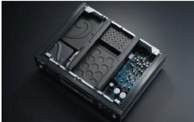
**6-Layered Main Circuit Board for High S/N Ratio**
