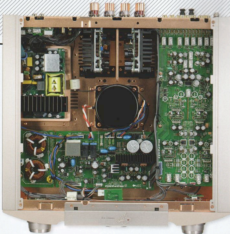
ABOVE: Marantz's MMP phono stage and HDAM-SA3 preamp section occupies a full third of the amplifier [right] while a small toroidal transformer [centre] feeds both linear [bottom] and switchmode PSUs [top left], the latter for the pair of Hypex power amp modules [top centre]
