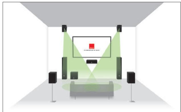
DALI ALTECO C-1 placed high on the front wall in a 5.1.2 surround system for height information.
