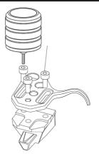
Rega's custom cartridge torque wrench is designed to apply accurate and even torque (0.4Nm) to each mounting bolt ensuring optimum performance. Fit all three mounting bolts then tighten each one fully until the tool 'clicks' three times. Only use the supplied mounting hardware.
