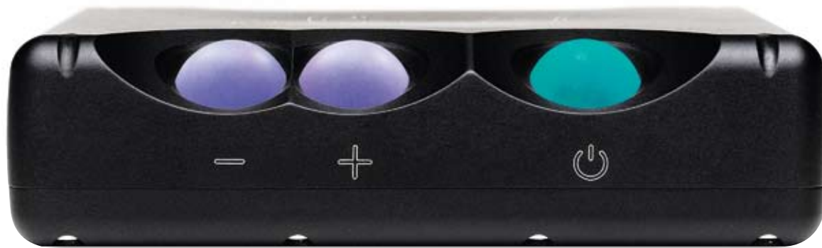
LEFT: The Mojo has Chord's usual 'milled from solid' aluminium casework for durability, while the single power button lights to indicate digital lock, and changes colour to show sample rate
