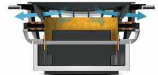
Blade driver with a vented coupler
