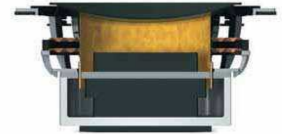
Conventional driver traps air inside
