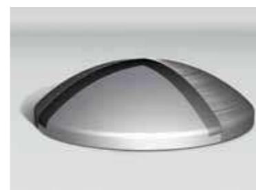
The tweeter has a two-part dome construction that forms a triangular strut to increase rigidity
