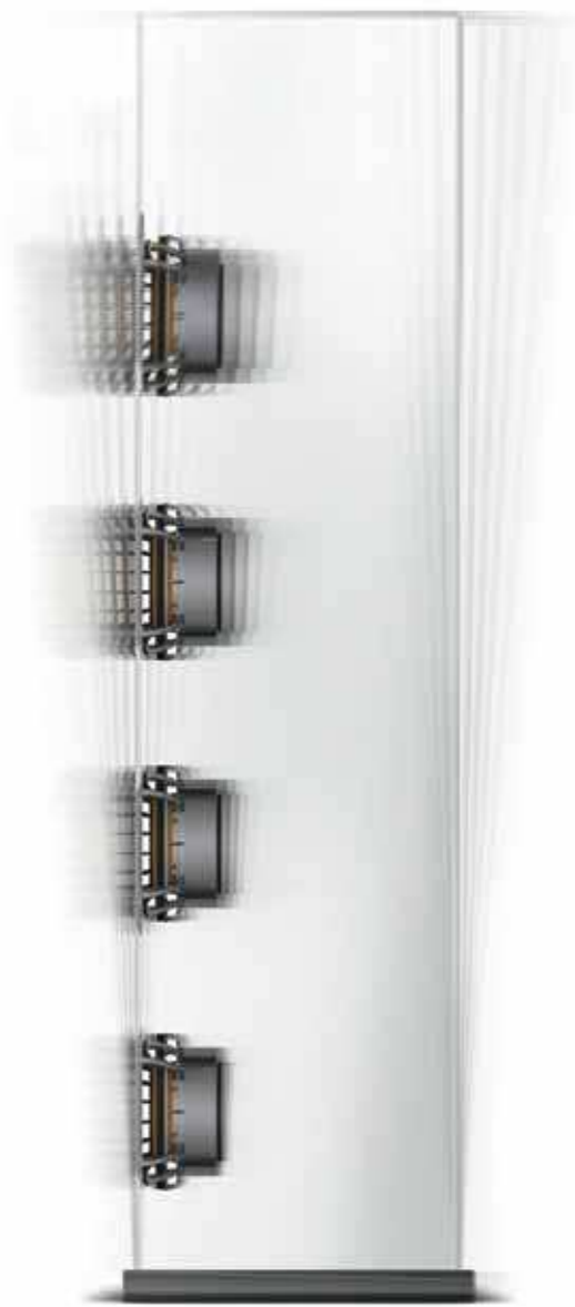
Conventional speaker generating cabinet resonance
