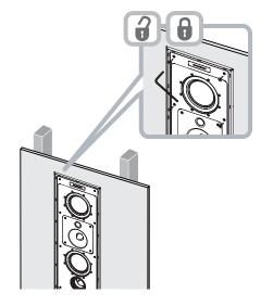
**4.7** The baffle can now be inserted into the back box. The baffle insertion and attachment technique is slightly different in the case of the CWM7.3 and CWM7.4/5. In both cases however you should first ensure that the connector on the baffle is oriented correctly with the connector inside the back box.
