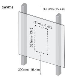
All CWM7 Series speakers require a clear depth of 102mm (4.02 in) from the front of the ceiling surface.
