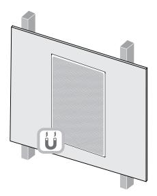
**4.9** The grille can now be fitted to the baffle. It is held in place magnetically so simply needs to be aligned with the groove in the back box flange where it will click into place. The diagram above illustrates fitting the grille.
