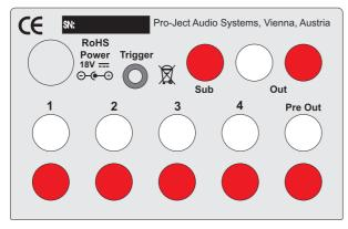
Make all connections whilst the preamplifier is disconnected from the power supply.
