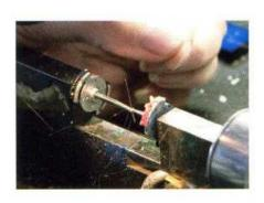
Winding of very small moving-coil armatures processed by hand under microscope - using copper-wires with a thickness like human hair.
