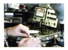
Final testing of each moving-coil cartridge by using several test-records and recording equipment.
